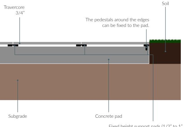
Fixed height support pads (1/2" to 1" high). The pedestals can be taken apart.
